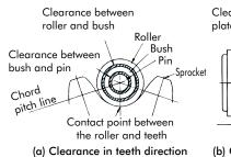
Clearance between roller link plate and teeth
