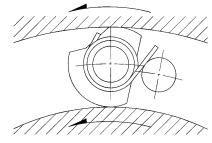
Figure 3: Inner and outterrace locked and turning
