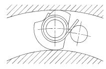
Figure 1: Entire Cam Clutch is stationary
