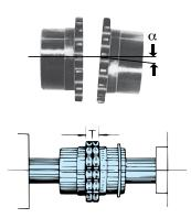
Place a straight edge at the bottom of corresponding teeth of the two sprockets and adjust so that parallel misalignment is minimized. Allowable parallel misalignment ( $\epsilon$ ) is 2% of the chain pitch.
