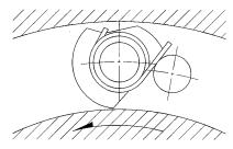
Figure 2: Inner race only turning
